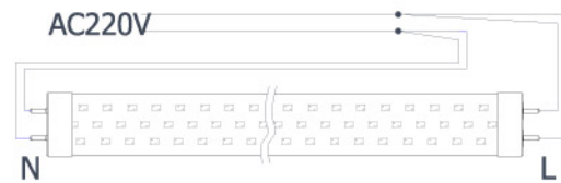
Connection diagram of a LED tube light
